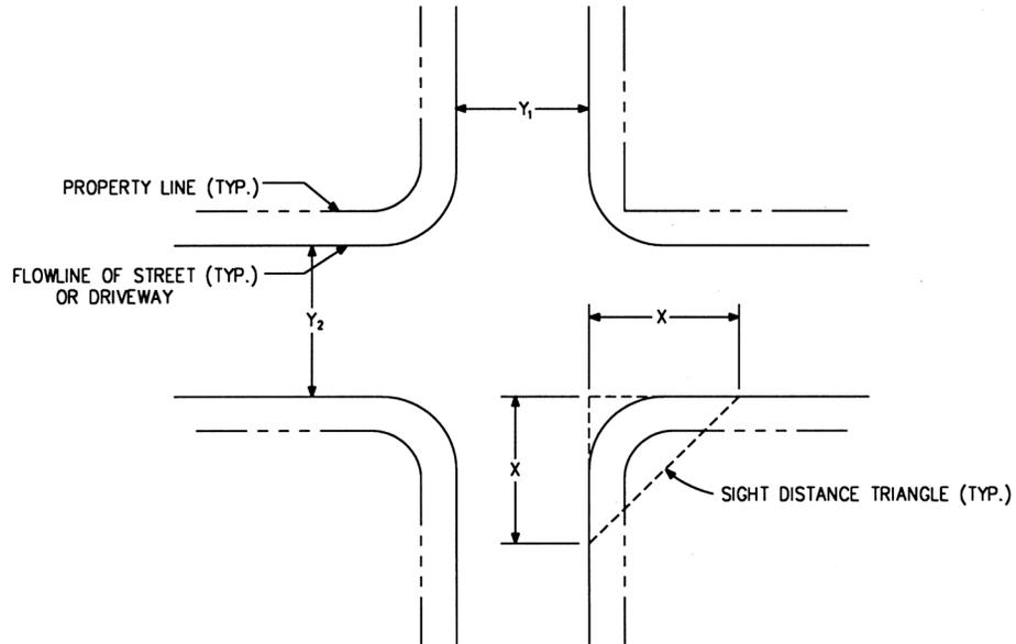
NOTE: IF  $Y_1 \neq Y_2$  USE THE LARGER OF THE TWO TO DETERMINE THE "LEG LENGTH" OF THE SIGHT DISTANCE TRIANGLE
