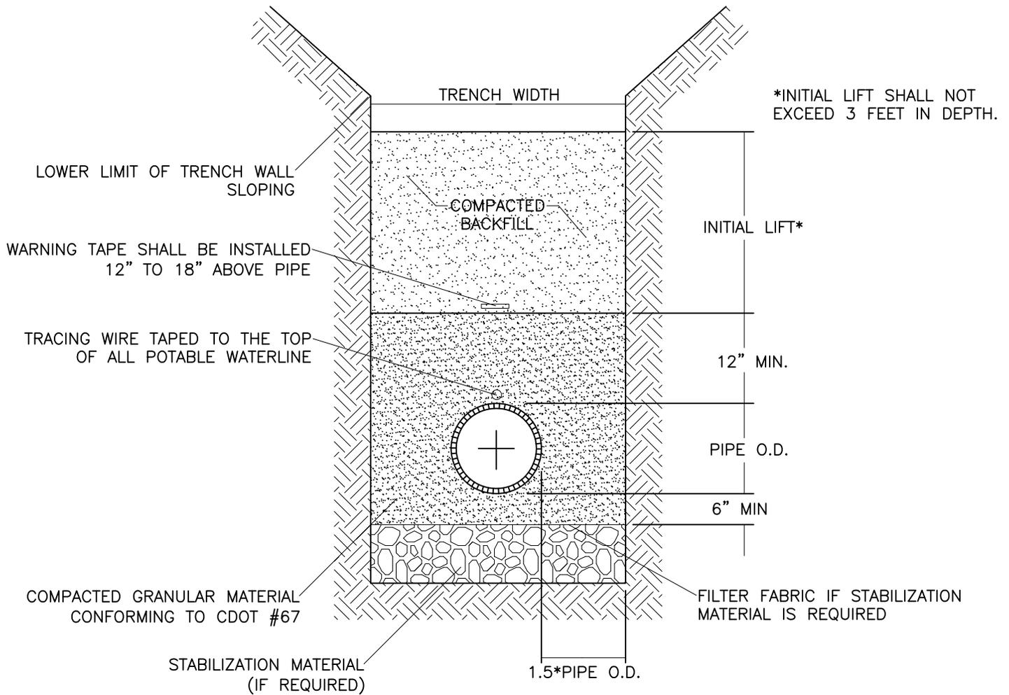
\*INITIAL LIFT SHALL NOT EXCEED 3 FEET IN DEPTH.
